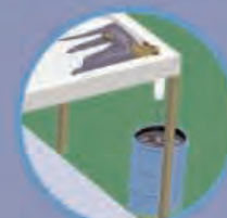
Flat roof without adequate drainage
